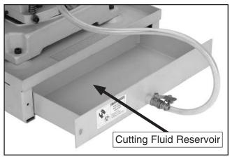
Figure 10. Cutting fluid reservoir.
